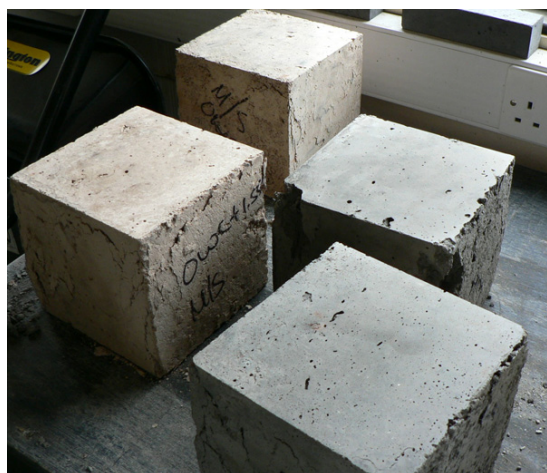
Figure 5 - HBM cubes and cores for testing
