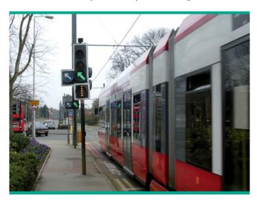
For trams at signal-controlled road junctions, signals to one of the variants of diagram 3013 of the  $TSRGD^6$  are used. The tram signals are often mounted alongside standard signal displays as shown in  $TSRGD^6$ . Facilities for pedestrians crossing at signal-controlled junctions and elsewhere on the system need to be considered at the start of the project.
