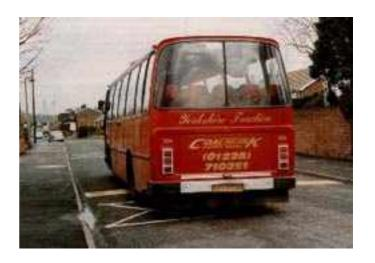
A track trial was conducted by TRL. 50mm high by 900mm wide thumps were used at 25m intervals. These were slightly higher than those in Wakefield, but conformed to the minimum height allowed under the road humps regulations.
