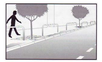
This is an open railing, constructed from a continuous 50mm diameter tubing, to form unit 1.5m to 2.5m long. and а approximately 1m in height. Gaps, no wider than 1.5m, are provided between individual units to allow pedestrian movements. Visually impaired cane users
