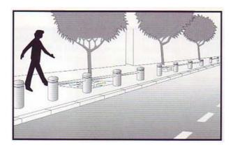
These consist of railing no more than 0.5m high, supported by posts 3m apart. The posts will generally not be more than 0.9m high. Gaps can be left for pedestrian use, but the low height of the railing may cause difficulties for visually impaired people. This type of fencing is generally best when used in conjunction with landscaping where the aim is to keep pedestrians away from the carriageway.
